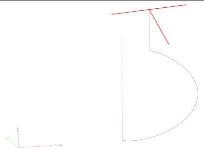
Figure 2-2: Helical interpolation example toolpath
