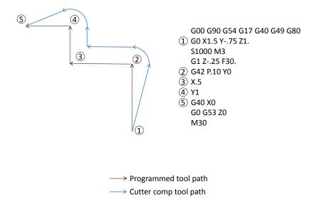
Figure 41-7: G42 cutter compensation path.
