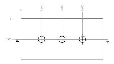
Figure 90-1: Hole pattern example
