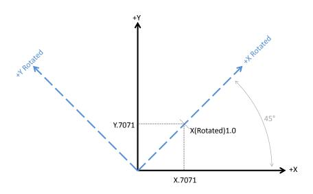
Figure 68-1: Coordinate system rotation (G68 X0 Y0 R45)
