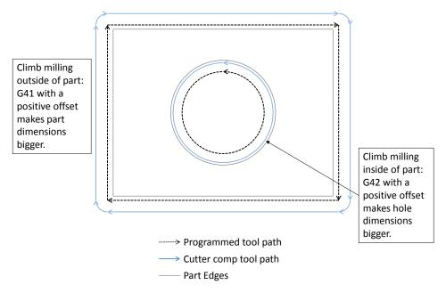
Figure 41-2: Cutter compensation OD and ID features.
