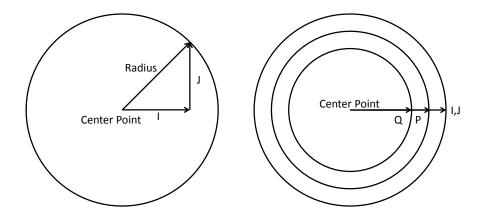
Figure 12-1: Tool motion during circle interpolation
