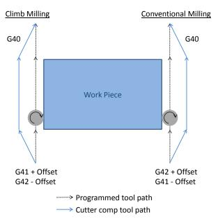
Figure 41-1: Cutter compensation offset direction.
