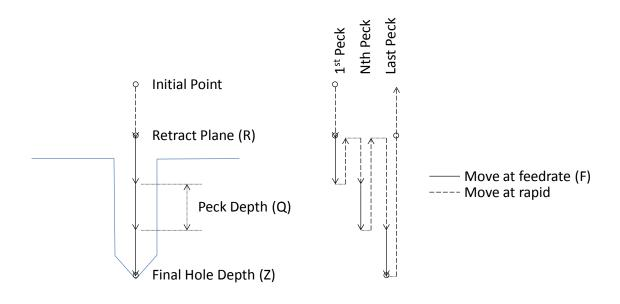
Figure 83-1: Motion of tool point for G83 cycle. End Z position will be determined by G98/99 setting.
