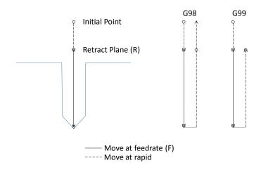
Figure 98-1: Initial and R point return setting.
