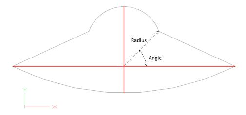
Figure 15-1: Tool path of polar coordinate mode example
