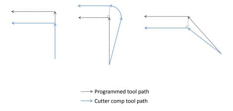
Figure 41-3: Cutter compensation start blocks.
