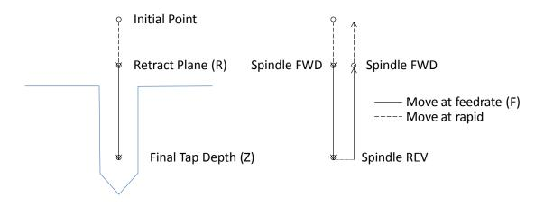
Figure 84-1: Motion of tool point for G84 cycle. End Z position will be determined by G98/99 setting.
