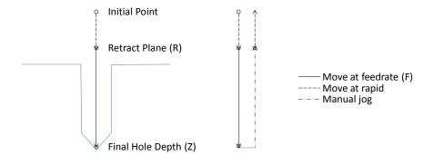
Figure 88-1: Motion of tool point for G85 cycle.
