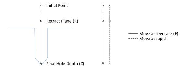
Figure 81-1: Motion of tool point for G81 cycle. End Z position will be determined by G98/99 setting.
