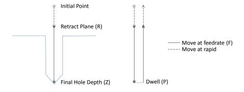
Figure 89-1: Motion of tool point for G89 cycle. End Z position will be determined by G98/99 setting.
