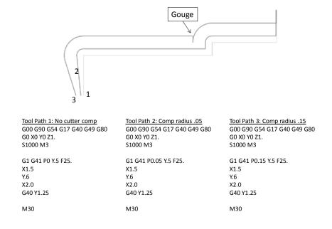
Figure 41-4: Cutter compensation radius and gouge.
