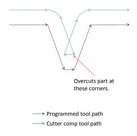
Figure 41-5: Cutter compensation in narrow groove.
