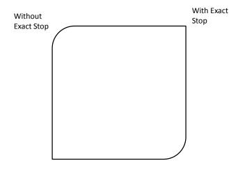
Figure 9-1: Square with exact stop on two corners
