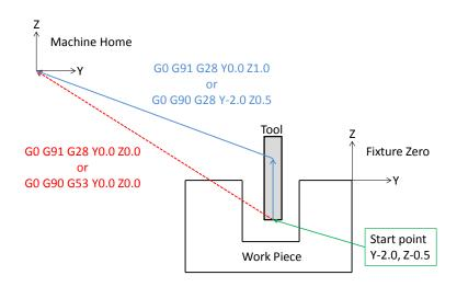
Figure 28-1: Zero return via intermediate point
