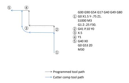
Figure 41-6: G41 cutter compensation path.
